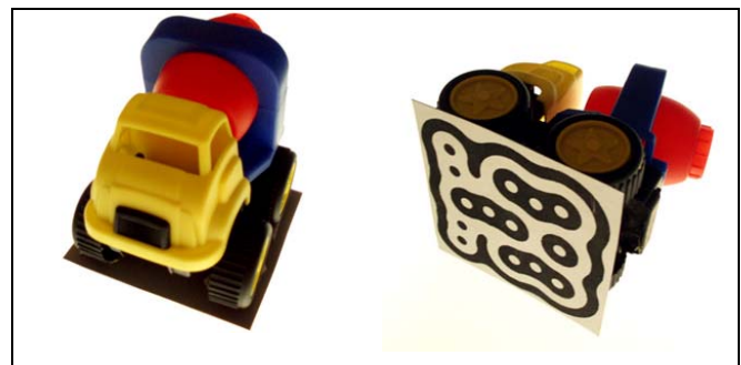
Figure 7 – images of the car used in the prototype, with a fiducial tag attached underneath
